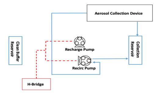
The two-pump system continuously circulates the buffer fluid to concentrate particles. The H-bridge is used to reverse the polarity to drain the fluid lines into the collection reservoir at the end of the cycle.
