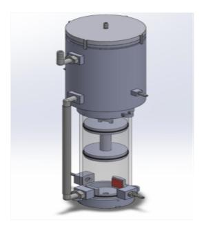
Submersible water activity meter CAD drawing showing the syringe concept
