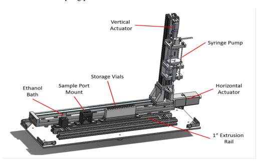
The syringe tower includes a vertical actuator and a syringe pump. In this example, the tower is coupled to a horizontal actuator that is configured to move a storage vial, a sample port mount, and an ethanol bath along an extrusion rail.
