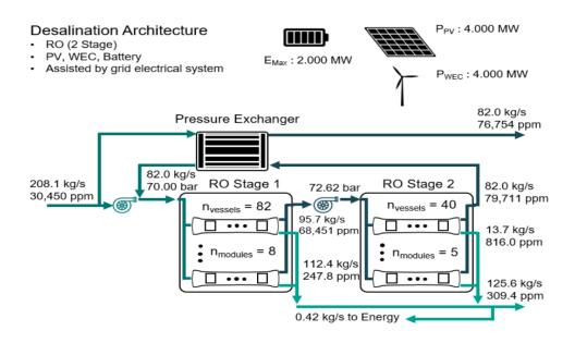
Example diagram of optimal architecture based on selected attributes
