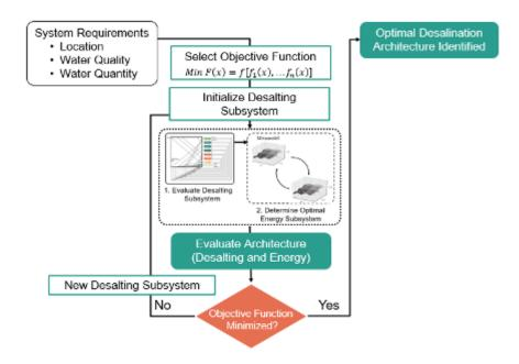
Basic optimization structure for evaluating complete desalination architectures
