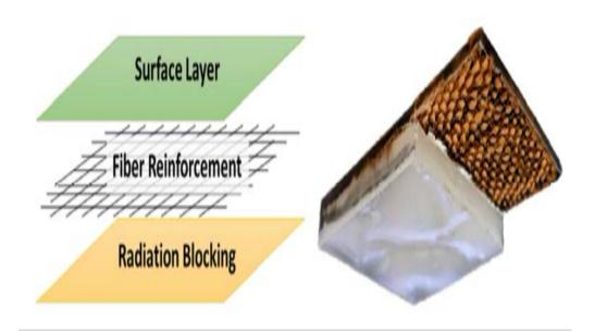
Schematic of multi-layer composite structure with distinct surface, fiber reinforcement, and bulk layers (left) with a prototype sample constructed of rGO-dd and HDPE as the surface layer with Zylon reinforcement and HDPE backing layer (right)
