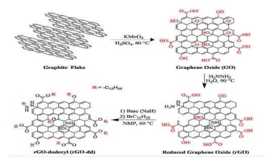
Schematic of rGO functionalization scheme to form rGO-dd. In this depiction, the process starts with commercially purchased graphite flake that is exfoliated using the Hummer's method; however, the scheme is compatible with many rGO production methods. Functional groups in red are highlighted for clarity in following the reaction sequence.
