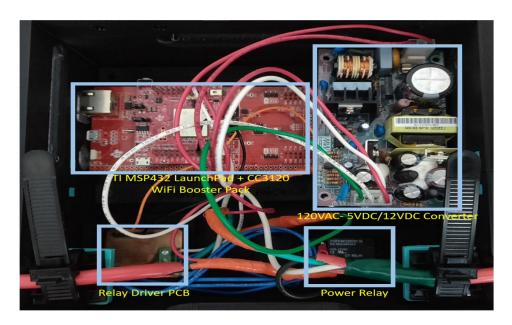
Modules inside the final prototype.
