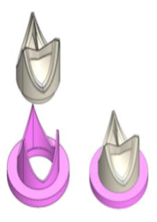
Example of 3D-printed valve assembly where the leaflet portion (beige) can be easily mounted on top of the frame (purple).
