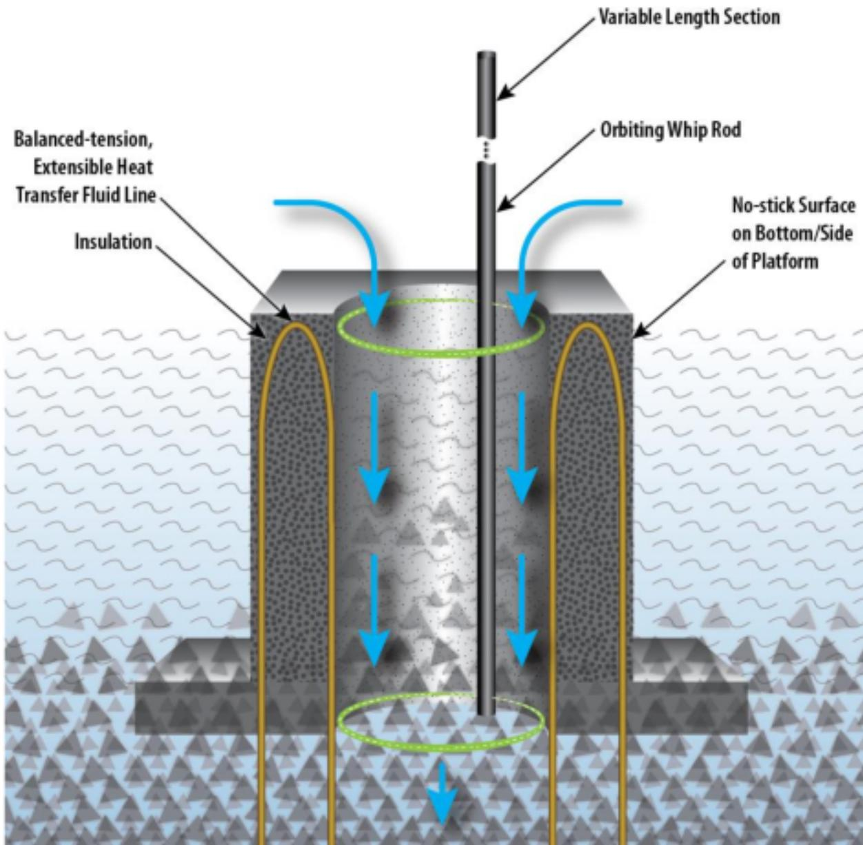
This vertical cross-sectional concept of Georgia Tech's buoyant platform during thermal discharge illustrates how liquid PCM flow is induced in a relative downward manner as a whip rod facilitates solidification. The platform passively elevates to remain above the bulk solid/slurry front, given engineered buoyancy. Solid PCM is indicated by the triangles shown collecting at the bottom, and liquid PCM is indicated by the wavy lines toward the top.
