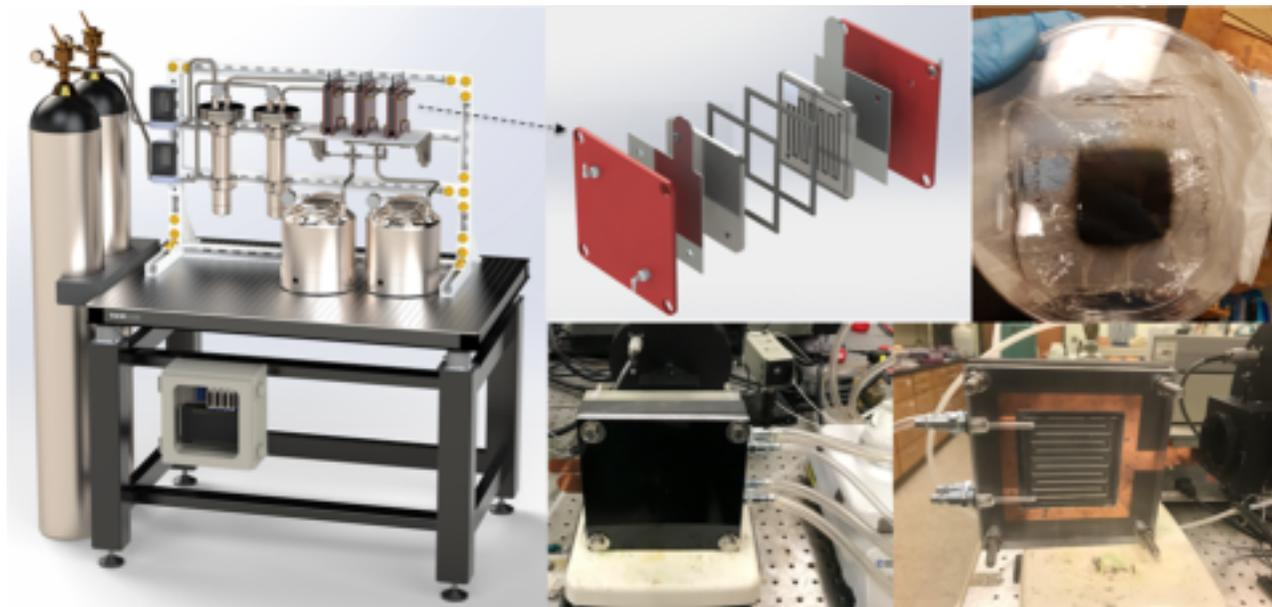
Schematic of the gas-phase (photo) electrochemical cell for nitrogen fixation using hybrid plasmonic nanocages. (center top) In this setup, the catalyst materials are painted on both sides of the membrane surface, as shown in the top right image. Note that the generated ammonia in the gas form will be liquefied using the condenser as depicted on the benchtop.
