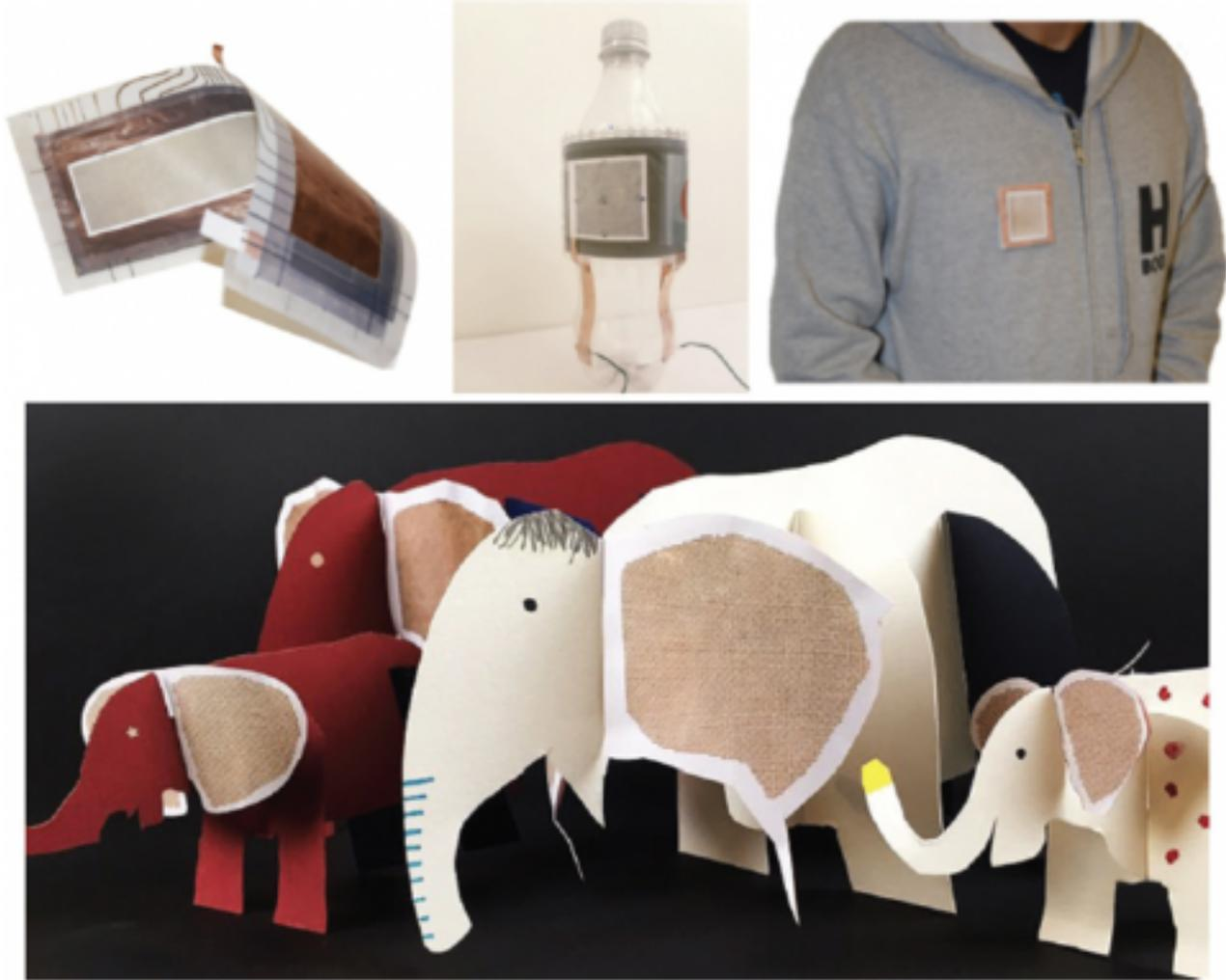
SATURN is flexible and can be made in different shapes and sizes, allowing instrumentation of everyday objects such as a soda bottle, shirt, and paper crafts.
