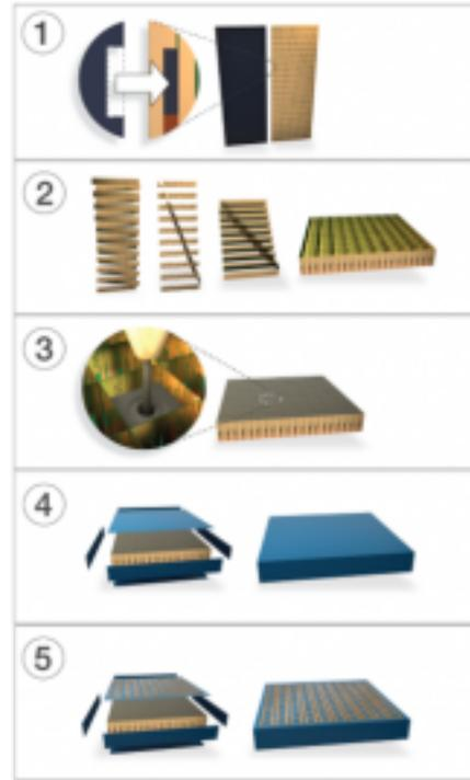
Printed circuit board panel with unit cells array (left). Multi-step construction process resulting in 3D unit cells with resonant element decorating the sidewalls, structural fillers, novel material systems, dielectric skins, and 2D arrays (right). The resulting composite is a structural laminate with a tailored EM response.
