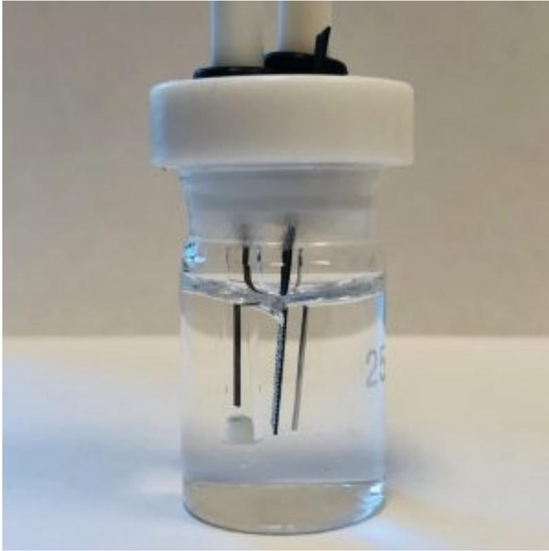
Electrochemical lithium extraction cell. Photo by Po-Wei Huang
