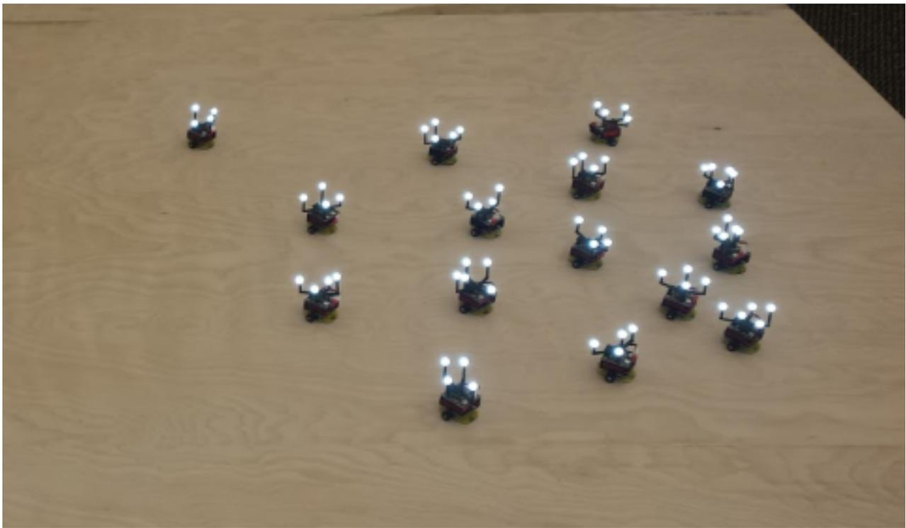
An example of a small robot swarm that could be guided through this method
