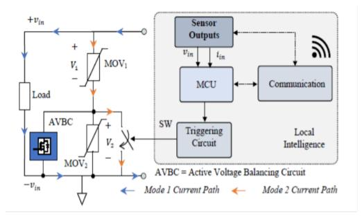
High-level electrical schematic of the system.
