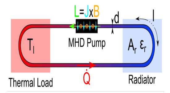
Schematic representation of the liquid metal loop
