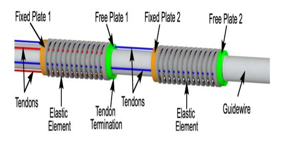
Example 1: Two compression springs are discretely located at two separate sections of the guidewire - combination of fixed plate and free plate at either end of the spring will enable tendon routing and termination.
