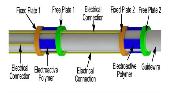
Example 2: A representative EAP element is shown at the location where stiffening is desired in the guidewire. The electrical wires would be routed similarly as the tendon(s)/push rod(s) to independently actuate each EAP element.
