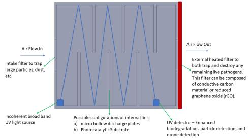
Air Purification System Diagram
