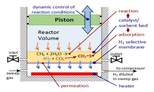
Schematic shows the components of a CHAMP cylinder-piston assembly used to create hydrogen from methane and steam via variable volume catalytic reaction. The process also concentrates carbon dioxide emissions from the process. (Credit: David Anderson, Georgia Tech)
