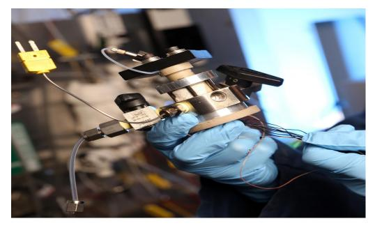
Georgia Tech researchers have demonstrated a CHAMP reactor, which uses the four-stroke engine cycle to create hydrogen while simultaneously capturing carbon dioxide emission. (Credit: Candler Hobbs, Georgia Tech)
