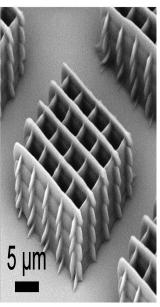
3D printing with submicrometer features through projection of arbitrarily patterned temporally focused femtosecond light sheets. Printing errors can be minimized by appropriately structuring the digital masks and controlling the projection sequence.
