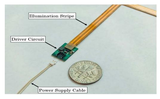
The system's small-form driver circuit and illumination stripe connecting to the power supply
