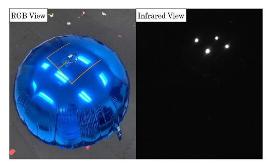
The active marker installed on a miniature autonomous blimp; the markers are highly conspicuous in the infrared view
