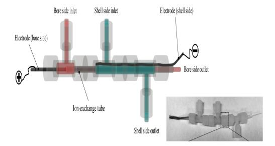
Tubular design of the power module.
