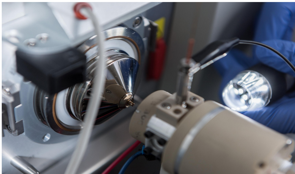
The DRILL device connected to a mass spectrometer in the Georgia Tech lab
