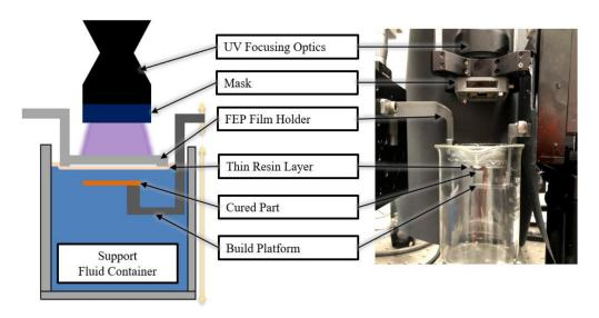
Setup of the fluid interface-supported printing system
