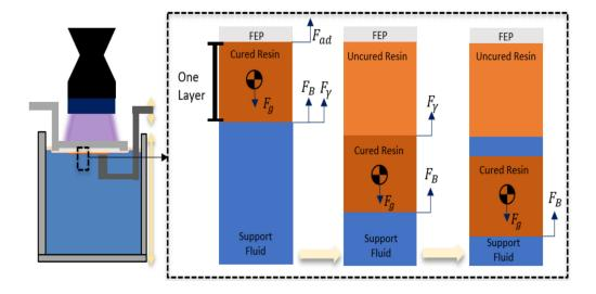
Diagram showing the forces associated with the removal of a cured layer from the FEP film
