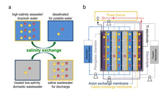
Salinity exchange a) Schematic of the salinity exchange concept and b) operation of a salinity exchange electrodialysis (SEE) system.
