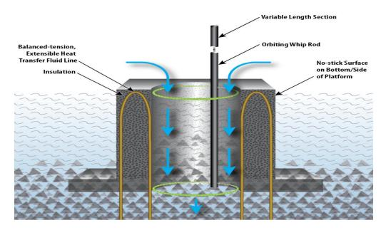
This vertical cross-sectional concept of Georgia Tech's buoyant platform during thermal discharge illustrates how liquid PCM flow is induced in a relative downward manner as a whip rod facilitates solidification. The platform passively elevates to remain above the bulk solid/slurry front, given engineered buoyancy. Solid PCM is indicated by the triangles shown collecting at the bottom, and liquid PCM is indicated by the wavy lines
