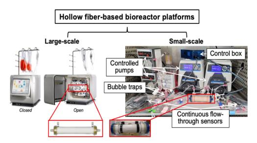
"Smart" hollow fiber bioreactor with in-line sensors informing feedback controls for autonomous feeding and regulation of culture environment.
